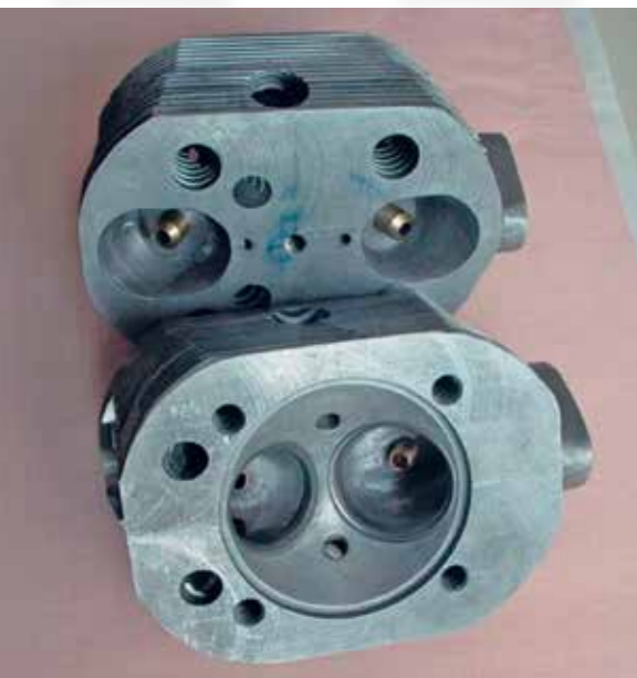
Zylinderkopf, E = 49 mm, A = 43 mm (P. Pohl)
